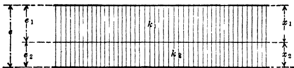
FIG. 14.—Dielectrics of different permittivities in series.
